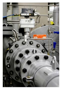
IGVs retrofitted onto an existing Sundyne multi-stage compressor.
