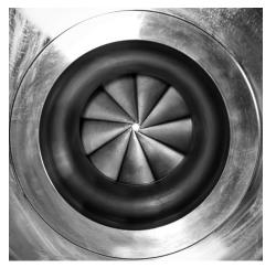
IGV blades at the inlet of a compressor pre-swirl gas flow entering the impeller, which reduces the amount of work needed from the main driver.
