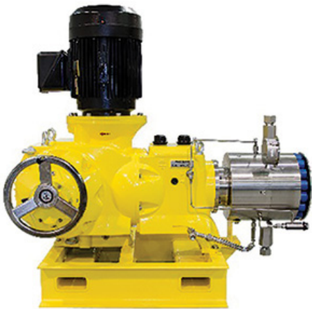
This specialized metering pump features a vertical motor configuration and metallic liquid end with metallic double diaphragm. The pump is designed for pressures up to 1,380 bar.
