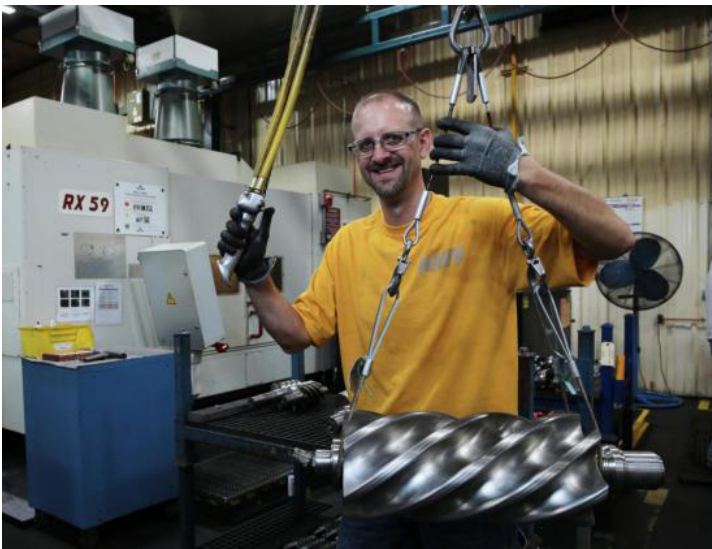
Sullair’s factory in Michigan City has a rich technical heritage manufacturing a wide range of rotary screw compression technologies including gas, two-stage, low-pressure, vacuum, and single-stage airends.
